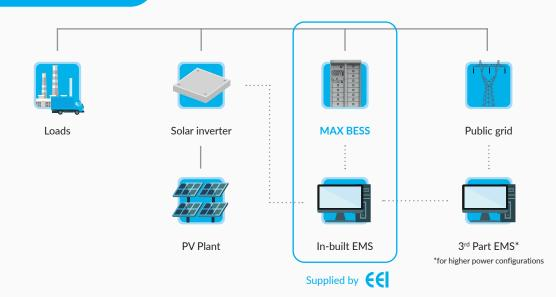
EEI Max BESS allows to be easily integrated in on-grid systems as an All-in-one Energy Storage unit, reducing at maximum all efforts needed to integrate different type of batteries, BMSs and PCSs. The fast and intuitive installation permit to easily integrate energy storage in your plant and immediatly benefit from all the in-built functionalities of EEI Max BESS.
